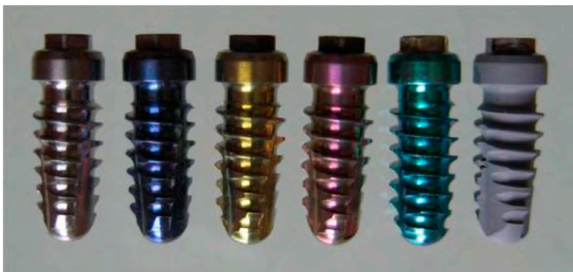
Figure 6. Uncoated Ti cp with colorless native oxide film, from blue to green, the electric-potential-dependent anodic pre-spark films, and the gray surface of an anodic spark-discharge-generated coating (left to right). Reproduced with permission [319].
