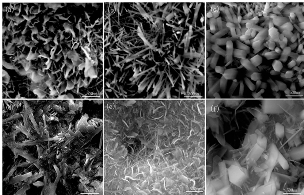
Figure 15. SEM images of different HA structures after MAO hydrothermal treatment for 6 h ((a) 150 °C, (b) 200 °C, and (c) 250 °C, (d) 250 °C—6 h in 100 mL solution, (e) 250 °C—6 h in 400 mL solution; (f) 250 °C—12 h in 200 mL solution). Reproduced with permission [367].
