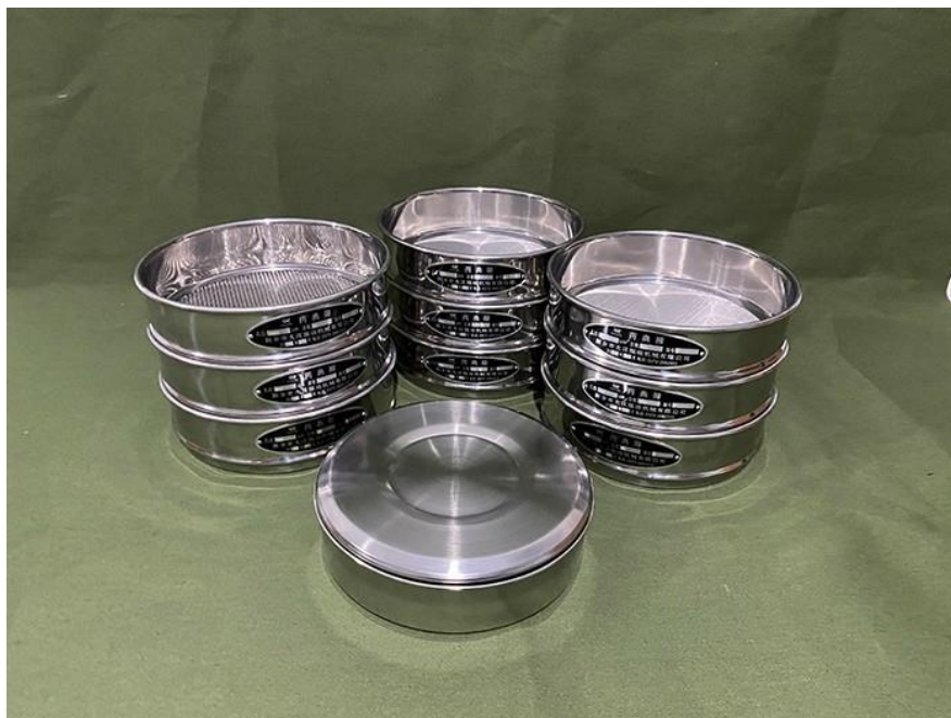
Img. 14. Sieves for testing distribution of powder particles by size (site:images.google.com)
