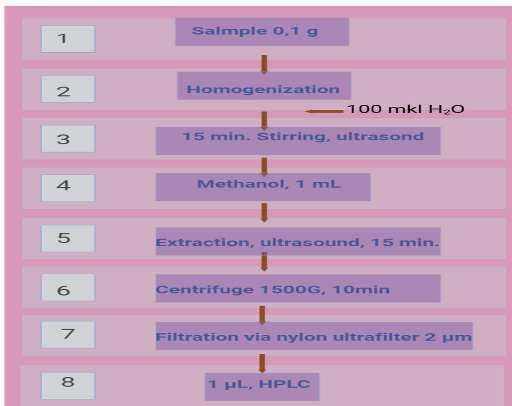
Figure 2. The sample preparation technique
