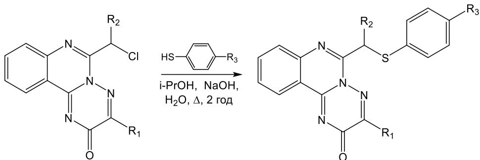
R<sub>1</sub> = Ph, 4-i-PrC<sub>4</sub>H<sub>6</sub>, 4-F-Ph; R<sub>2</sub> = H, Me; R<sub>3</sub> = H, Me, Cl, F
